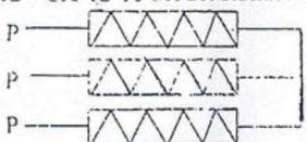
4. SRJX-2-13 SRJX-2.5-13 Model The carbon stick of silicon connect method sketch map
