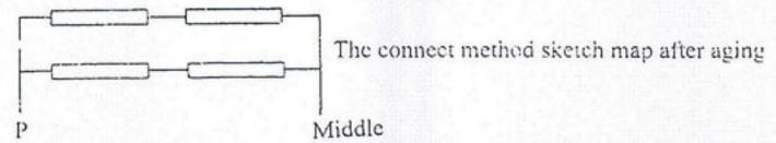
5. SRJX-4-13 SRJX-5-13 Model The carbon stick of silicon connect method sketch
