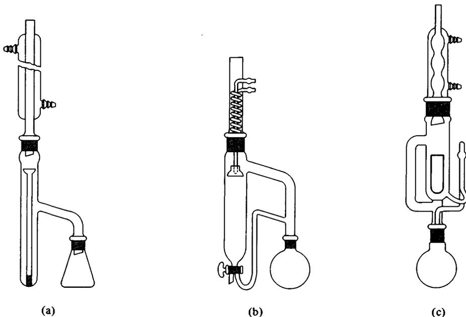
FIG. A3.11. Continuous extraction setups (a) for solvents less dense than water (b) for solvents more dense than water (c) Soxhlet extractor.
