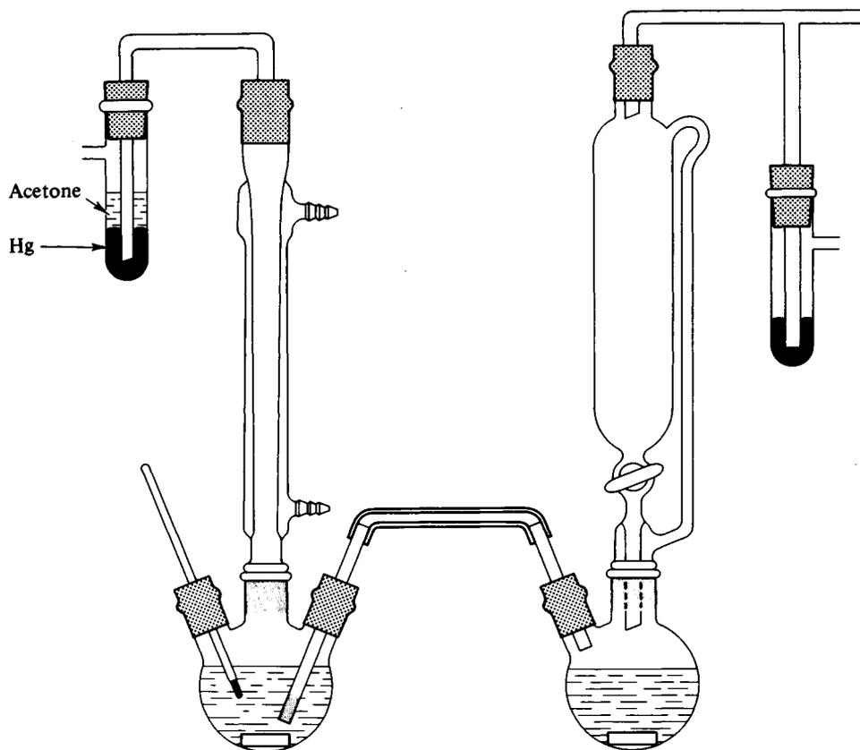
FIG. 4.1. Apparatus for the external generation of diborane.
