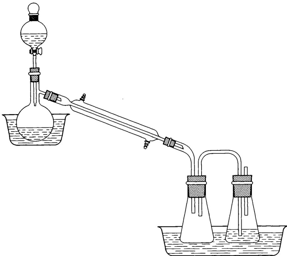
FIG. 17.1. Apparatus for the generation of diazomethane.
