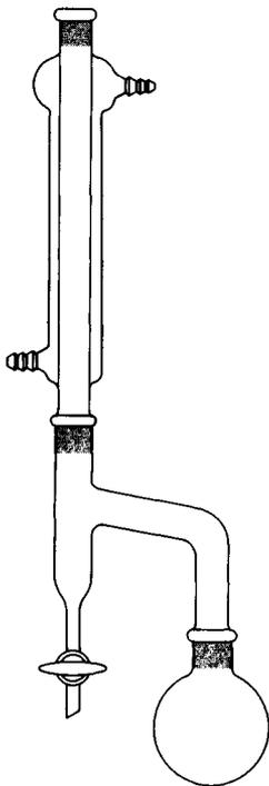
FIG. A3.6. Dean-Stark trap for continuous removal of water.
