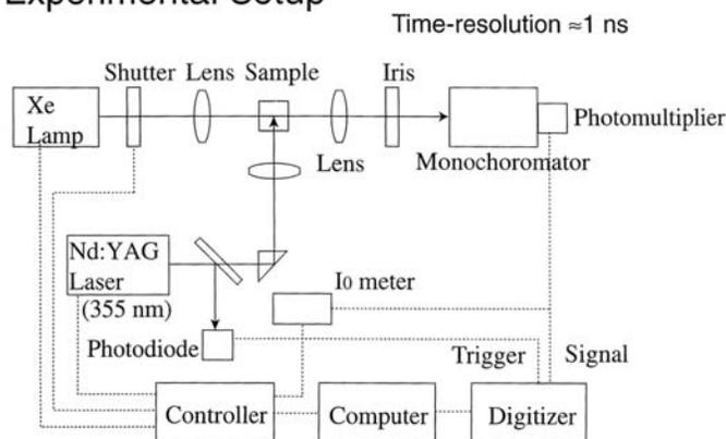
Diagram of laser flash photolysis apparatus
